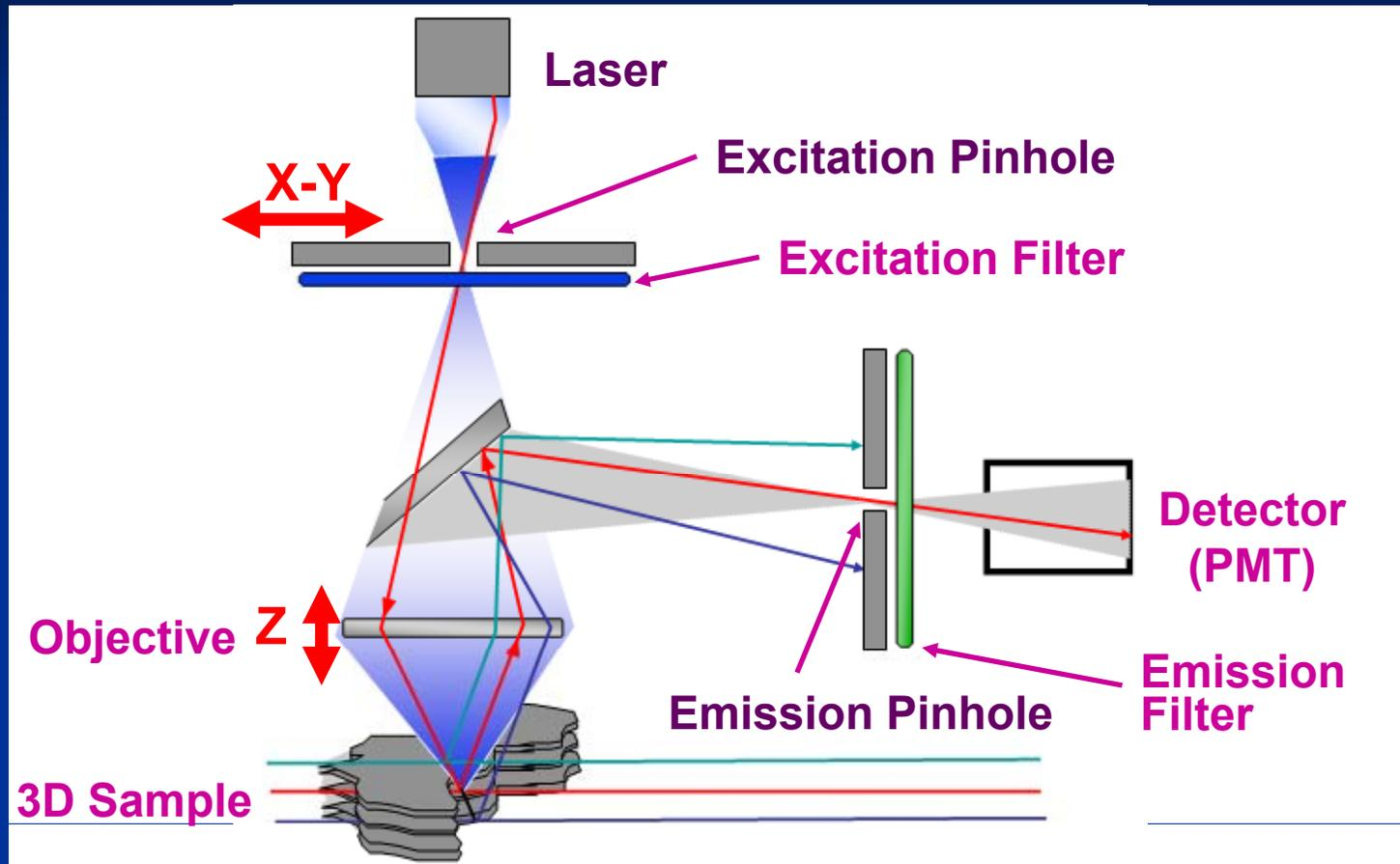
A type of light microscopy in which a point of illumination is projected or rastered over a specimen, and the reflected illumination is screened through an exit aperture in order to eliminate light from out-of-focus planes.
