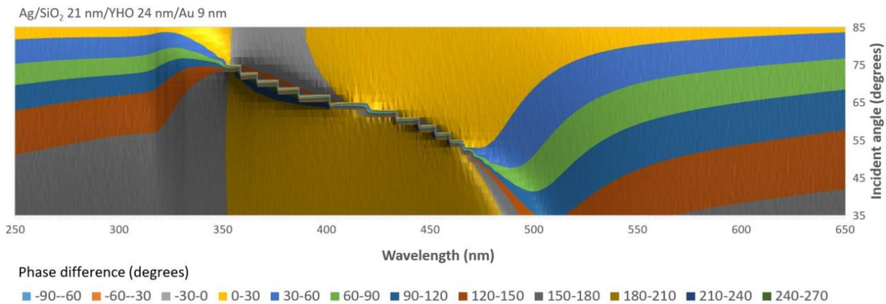
**Figure 3.** The 3D representation for the phase difference of  $p$  and  $s$  polarized light as a function of wavelength and incident angle of light. Multiple phase-singularities (between  $-90^\circ$  and  $+270^\circ$ ) for multilayer structure of Ag/SiO<sub>2</sub>/YOH/Au at broad spectral range (~350-465 nm) for various incident angles (~55-75 degrees).
