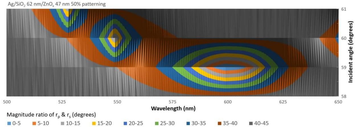
**Figure 1.** The 3D representation for the ratio of the reflection coefficients  $r_p$  and  $r_s$  for  $p$  and  $s$  polarized light as a function of wavelength and incident angle of light. No reflection of light for patterned ZnO<sub>x</sub> thin film at ~600 nm and at 59 degrees of incident angle.
