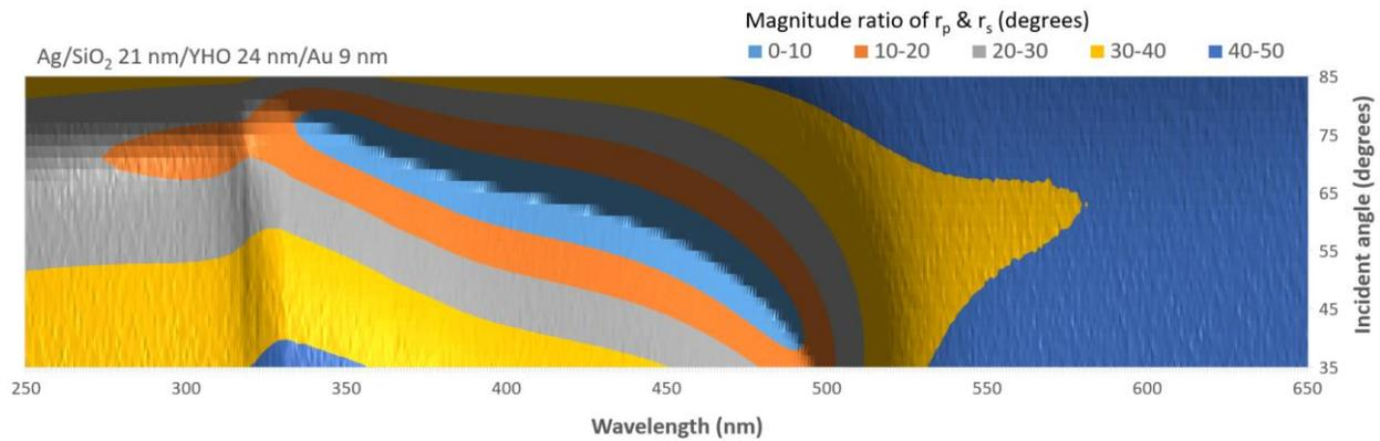
**Figure 2.** The 3D representation for the ratio of the reflection coefficients  $r_p$  and  $r_s$  for  $p$  and  $s$  polarized light as a function of wavelength and incident angle of light. No reflection of light for multilayer structure of Ag/SiO<sub>2</sub>/YOH/Au at broad spectral range (~340-490 nm) for various incident angles (~36-75 degrees).
