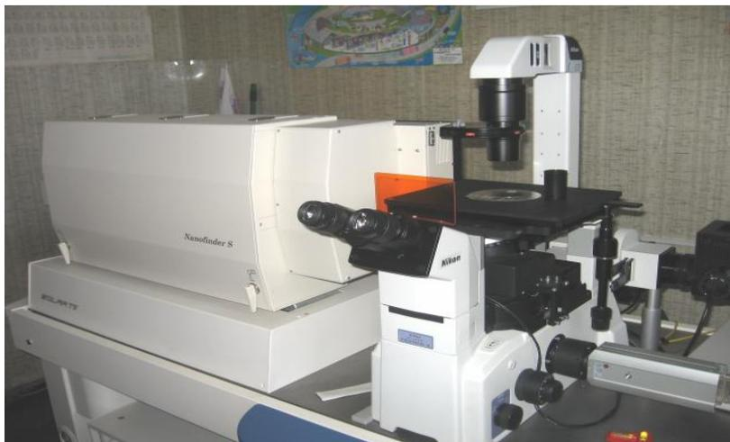
Fig. 2. "Nanofinder S" 3D Scanning Confocal microscope with Spectrometer
