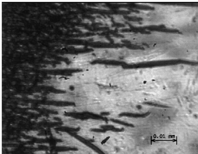
Fig. 3. The crystal surface after neutron irradiation without electric field. Distance between two vertical lines is equivalent to 0.01 mm.
