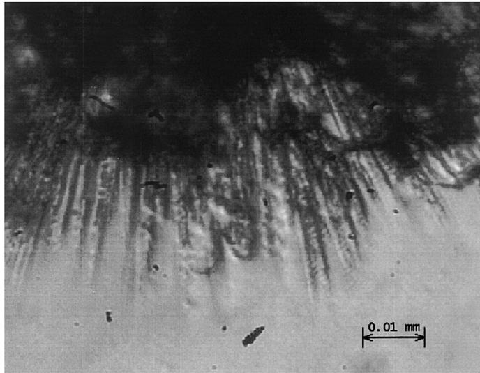
Fig. 4. The crystal surface after neutron irradiation with electric field. Distance between two vertical lines is equivalent to 0.01 mm.
