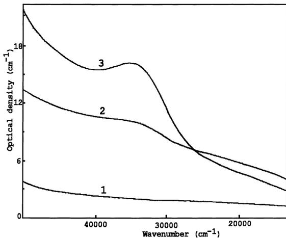
Fig. 2. The optical absorption spectra of lithium tetraborate. 1: before irradiation, 2: after irradiation of thermal neutron fluence  $10^{16} \text{ cm}^{-2}$  in electric field, and 3: after irradiation of thermal neutron fluence  $10^{16} \text{ cm}^{-2}$  without electric field.
