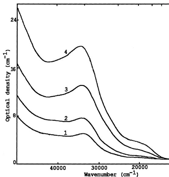
Fig. 1. The optical absorption spectra of neutron irradiated of fluence  $5 \times 10^{16}$   $\text{cm}^{-2}$  lithium tetraborate. 1:  $T = 444$  K with cadmium filter. 2:  $T = 444$  K without cadmium filter. 3:  $T = 300$  K with cadmium filter. 4:  $T = 300$  K without cadmium filter.
