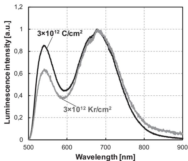
Fig. 2. The wavelength dependence of normalized luminescence intensity of  $\text{F}_3^+$  (530 nm) and  $\text{F}_2$  (670 nm) centers for LiF irradiated with 33.6 MeV  $^{84}\text{Kr}$  and 11.8 MeV  $^{12}\text{C}$  ions at fluence of  $3 \times 10^{12}$  ions/cm $^2$ . Excitation source: 473 nm laser.
