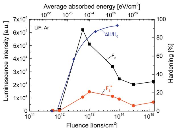
Fig. 6. Dose dependence of the hardening ( $\Delta H/H_0$ ) and luminescence intensity of  $F_2$  and  $F_3^+$  centers in LiF irradiated with  $^{40}\text{Ar}$  ions. Data from the profile curves (Figs. 3c,d and 4d) at a constant depth (11  $\mu\text{m}$ ).
