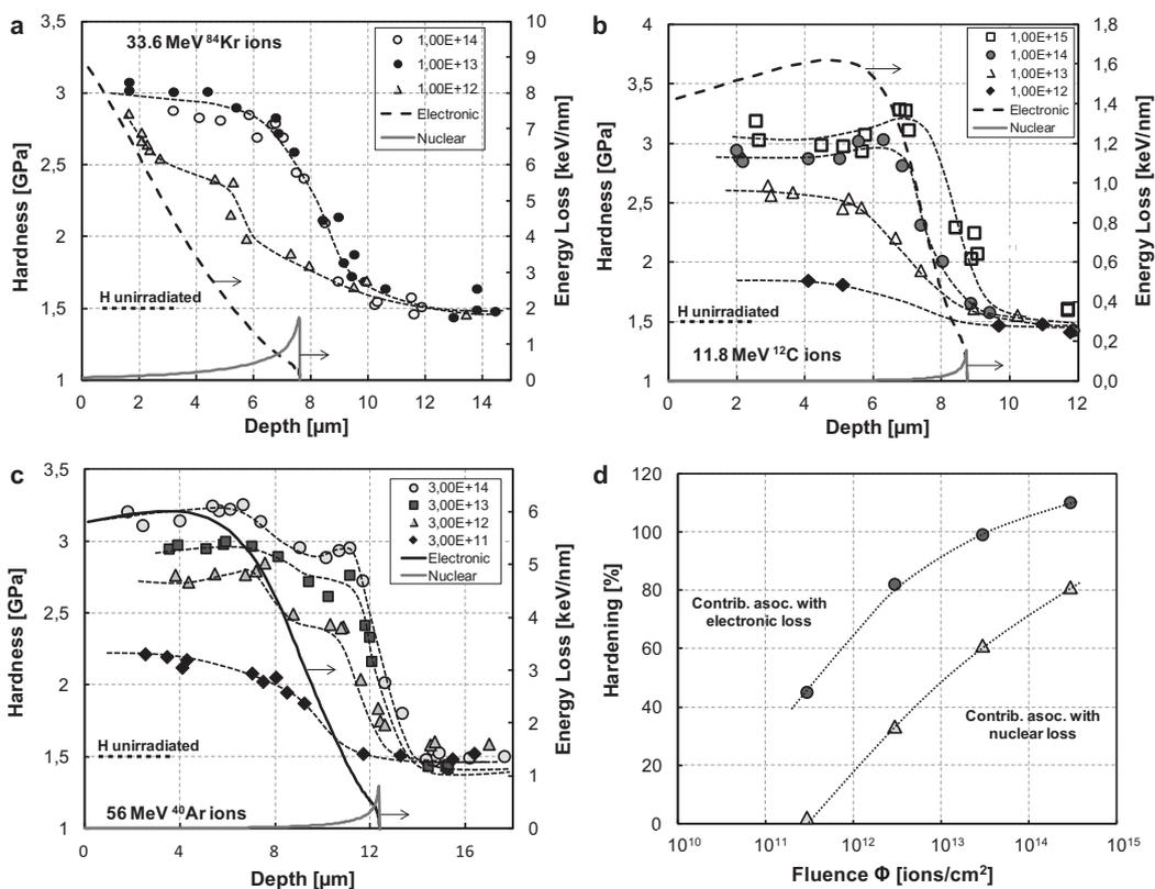
Fig. 4. Depth profiles of hardness in LiF crystals irradiated with (a) <sup>84</sup>Kr ions, (b) <sup>12</sup>C ions and (c) <sup>40</sup>Ar ions; (d) – dependence of hardening on fluence for <sup>40</sup>Ar ions at the depth of 4 μm, where the ion stopping is determined by electronic energy loss, and at 11.7 μm depth where dominates nuclear energy loss.
