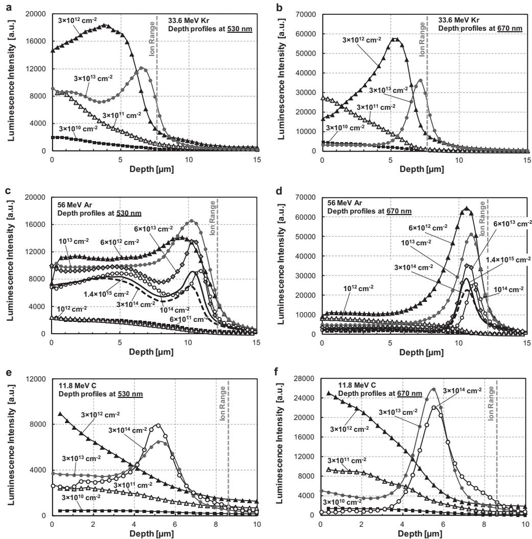
Fig. 3. Depth profiles of the luminescence intensity at 530 nm and 670 nm for samples irradiated with  $^{84}\text{Kr}$  (a, b),  $^{40}\text{Ar}$  (c, d) and  $^{12}\text{C}$  (e, f) ions at different fluences. The end of the range is marked with a dashed line.
