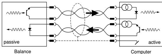
The passive current loops of the balance must be connected to external current sources. To avoid destruction of the CL interface by these sources, it is essential to observe the following limiting data:
