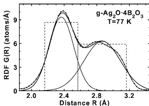
FIG. 7.  $G(R)$  of  $g\text{-Ag}_2\text{O}\cdot 4\text{B}_2\text{O}_3$  at  $T=77$  K determined by best fitting the EXAFS signal (full line with dots) and its approximation by a double Gaussian function (full lines without dots) and by a semiuniform distribution (dashed lines).
