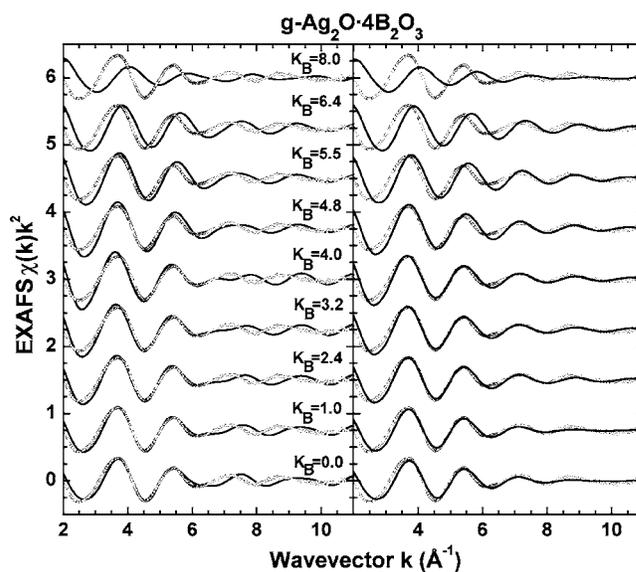
FIG. 9. Comparison between the experimental Ag  $K$  edge EXAFS of  $g\text{-Ag}_2\text{O}\cdot 4\text{B}_2\text{O}_3$ , measured at  $T=77$  K, with the theoretical EXAFS calculated for models conforming the semiuniform radial distribution (left panel) and conforming the double Gaussian distribution of Fig. 7 (right panel). The experimental signal is shown by open circles, the calculated signals are shown by full lines. The number of borons  $K_B$  is the same as in Fig. 8.
