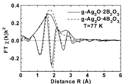
FIG. 3. Fourier transforms (FT) of experimental Ag  $K$  edge EXAFS signals in  $g\text{-Ag}_2\text{O}\cdot 2\text{B}_2\text{O}_3$  (full lines) and  $g\text{-Ag}_2\text{O}\cdot 4\text{B}_2\text{O}_3$  (dashed lines) at  $T=77$  K.
