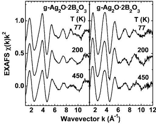
FIG. 2. Temperature dependence of experimental Ag  $K$  edge EXAFS signals  $\chi(k)k^2$  in diborate  $g\text{-Ag}_2\text{O}\cdot 2\text{B}_2\text{O}_3$  and tetraborate  $g\text{-Ag}_2\text{O}\cdot 4\text{B}_2\text{O}_3$  glasses.
