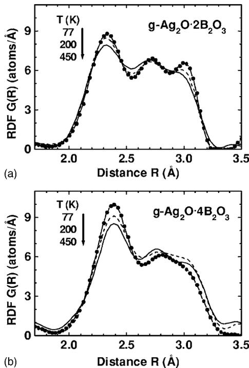
FIG. 6. Temperature dependence of the radial distribution functions  $G(R)$  in  $g\text{-Ag}_2\text{O}\cdot 2\text{B}_2\text{O}_3$  and  $g\text{-Ag}_2\text{O}\cdot 4\text{B}_2\text{O}_3$ , as determined from best fitting of the Ag  $K$  edge EXAFS.
