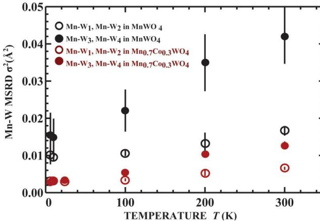
**Figure 5.** Temperature dependence of the MSRDR factors, obtained in RMC/EA simulations of  $\text{MnWO}_4$  and  $\text{Mn}_{0.7}\text{Co}_{0.3}\text{WO}_4$  for the Mn-W atom pairs along the crystallographic  $b$ - and  $c$ -axes.
