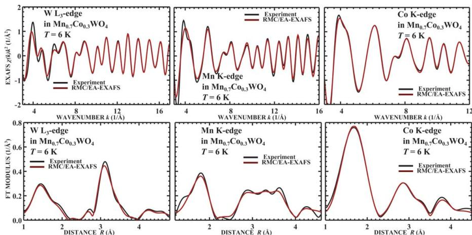
**Figure 3.** Comparison of the results of RMC/EA simulations (upper panels - EXAFS spectra, corresponding to the final structure model, bottom panels - moduli of their Fourier transforms (FT)) with the experimental W  $L_{3}$ -edge and Mn(Co) K-edges data for  $Mn_{0.7}Co_{0.3}WO_4$  at  $T = 6$  K.
