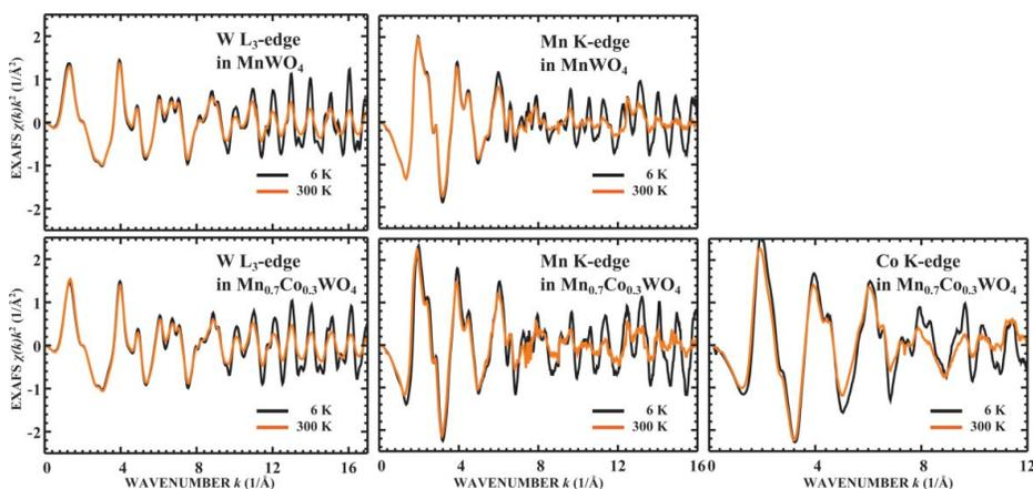
**Figure 1.** The experimental W  $L_3$ -edge (left panels) and Mn(Co) K-edges EXAFS spectra (middle and right panels) for  $\text{Mn}_c\text{Co}_{1-c}\text{WO}_4$  ( $c = 1.0$  and  $0.7$ ) at  $T = 6$  and  $300$  K.
