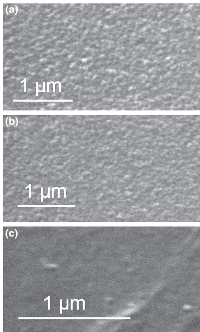
**Fig. 3.** SEM images of  $\text{Ni}_{1-x}\text{O}$  thin films simultaneously sputtered on (a) silicon, (b) glass and (c) polyimide film with  $\text{Ar}/\text{O}_2 = 90/10$ . Operating voltage was 25 kV.
