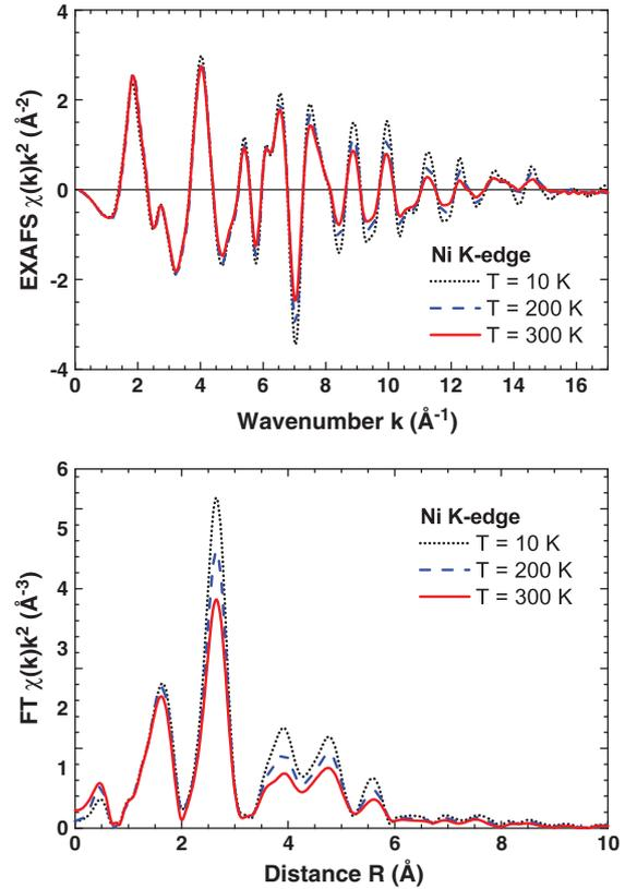
Fig. 5. Experimental Ni K-edge EXAFS spectra  $\chi(k)k^2$  and their Fourier transforms for the thin film TF3 ( $\text{Ar}/\text{O}_2 = 90/10$ ) at three selected temperatures. Note the EXAFS oscillations damping at high- $k$  values due to thermal disorder.
