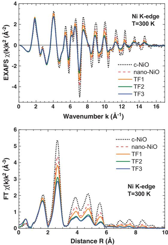
Fig. 4. Experimental Ni K-edge EXAFS spectra  $\chi(k)k^2$  and their Fourier transforms for the thin film samples compared with microcrystalline c-NiO and NiO nanoparticles (data taken from [18]). All data measured at  $T = 300$  K.
