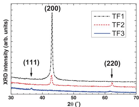
**Fig. 2.** XRD patterns of  $\text{Ni}_{1-x}\text{O}$  thin films prepared at three  $\text{Ar}/\text{O}_2$  gas ratios equal to 0/100 (TF1), 50/50 (TF2) and 90/10 (TF3).
