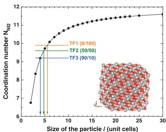
**Fig. 7.** Dependence of the average coordination number  $N_{\text{Ni}_2}$  in the second shell of nickel on the cubic nanoparticle size ( $L = l_{a_0}$ ). The parameters for three  $\text{Ni}_{1-x}\text{O}$  thin films are indicated. The inset shows the relaxed nanoparticle model with  $l = 3$  ( $3 \times 3 \times 3$  unit cells).
