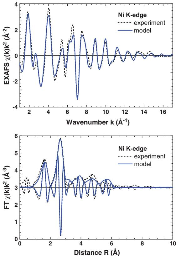
Fig. 8. Experimental (dashed line) and model (solid line) Ni K-edge EXAFS spectra  $\chi(k)k^2$  and their Fourier transforms for the film TF3 (Ar/O<sub>2</sub> = 90/10) at T = 300 K.
