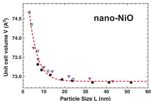
**Fig. 1.** Dependence of the unit cell volume on the nanoparticle size (data taken from XRD studies, solid circles from [12], empty circles from [13], empty box from [14], solid triangles from [15]). Dashed line corresponds to the fitted formula  $V = V_0 + A \exp(-L/B)$ , where  $V$  is the unit cell volume (in  $\text{\AA}^3$ ),  $L$  is the particle size (in nm),  $V_0 = 72.874 \text{ \AA}^3$ ,  $A = 3.9419 \text{ \AA}^3$ , and  $B = 3.8009 \text{ nm}$ .
