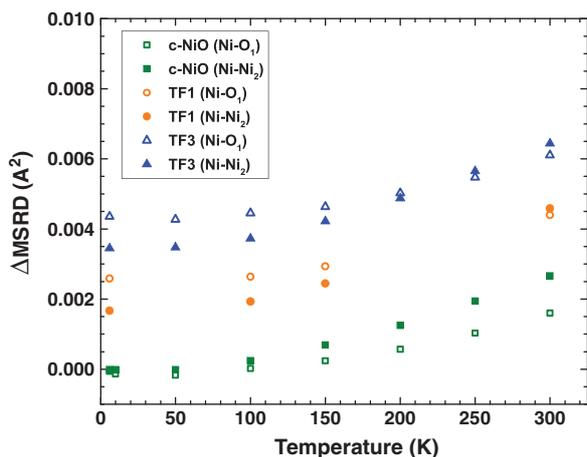
**Fig. 6.** Temperature dependence of the relative mean-square relative displacements ( $\Delta\text{MSRD}$ )  $\Delta\sigma^2$  for the first ( $\text{Ni-O}_1$ ) and second ( $\text{Ni-Ni}_2$ ) coordination shells in c-NiO and  $\text{Ni}_{1-x}\text{O}$  thin films relative to the MSRD value in c-NiO at  $T = 6$  K.
