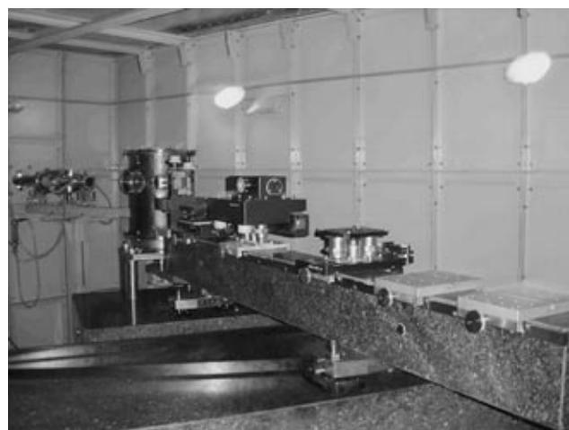
**Fig. 25.** Energy-dispersive EXAFS station: an X-ray monochromator, input X-ray optics, a mirror, and a detector are mounted on a granite mobile optical bench.
