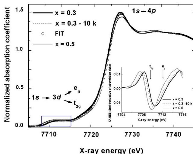
Fig. 5. Experimental (—) and calculated (o) Co *K*-edge XANES spectra for  $\text{La}_{1-x}\text{Sr}_x\text{CoO}_3$  ( $x = 0.3$  and  $0.5$ ) and multiple (10k) irradiated  $\text{La}_{0.7}\text{Sr}_{0.3}\text{CoO}_3$ .
