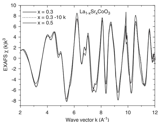
Fig. 3. Experimental EXAFS  $\chi(k)k^3$  signals at the Co  $K$ -edge in unirradiated  $\text{La}_{0.7}\text{Sr}_{0.3}\text{CoO}_3$  and  $\text{La}_{0.5}\text{Sr}_{0.5}\text{CoO}_3$  and multiple (10 k) irradiated  $\text{La}_{0.7}\text{Sr}_{0.3}\text{CoO}_3$  powders.
