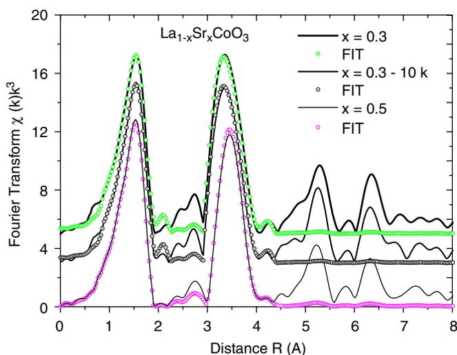
Fig. 4. Experimental (—) and fitted (o) Fourier transforms of the Co *K*-edge EXAFS  $\chi(k)k^3$  signals for the unirradiated  $\text{La}_{0.7}\text{Sr}_{0.3}\text{CoO}_3$  and  $\text{La}_{0.5}\text{Sr}_{0.5}\text{CoO}_3$  powders and ten-pulse (10k) electron-irradiated  $\text{La}_{0.7}\text{Sr}_{0.3}\text{CoO}_3$  sample.
